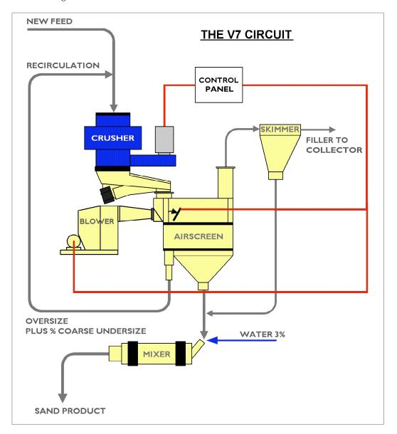
Once set to produce the desired gradation, the circuit is electronically controlled by reference to the crusher power consumption, and signals, to the damper and air screen blower, control the recirculation and filler extraction respectively, allowing a constant fineness modulus to be maintained.
