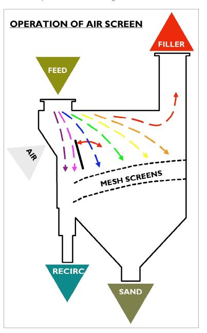
material to drop further along the screen chamber. An additional control, or damper, allows a proportion of the coarser particles to be diverted to recirculation, in order to control the top size and grading of the product within close tolerances. This feature allows the US7 crusher to produce the necessary amount of 150µm-1mm grains for an ideal particle size distribution. Fine filler is drawn off at the far end and is collected in a bag filter.
